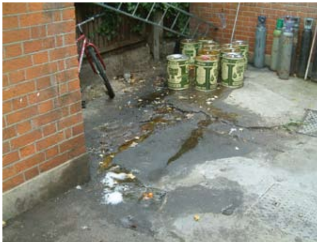
Avoid poor waste oil storage which could result in a sewer blockage or pollution incident.
